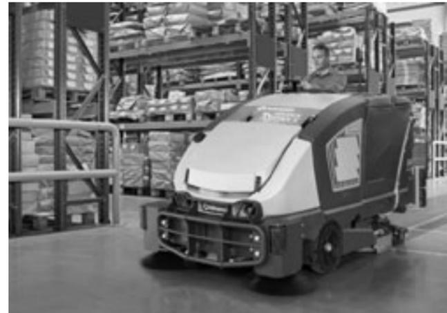
Operating solely on hydrogen, the Advance CS7000’s fuel cell is manufactured by Plug Power Inc. of Latham, New York. Featuring dedicated sweeping and scrubbing functions, the Advance CS7000 provides one-pass cleaning power for enhanced cleaning capabilities. Benefits include full operator shift of cleaning time between refuels; rapid refuel capabilities with no recharge cycle to enable 24/7 operation; and simple, two-connection setup for easy fuel cell installation.
