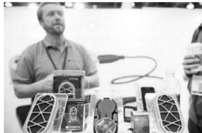
To use the \$229 PowerTREKK, you also have to purchase a \$4 PowerTREKK Pukk. Once you add a small amount of water (about half a shot), and add a one-time-use Pukk, the latter will immediately begin separating the hydrogen from the water, using it as fuel to charge your handset.
