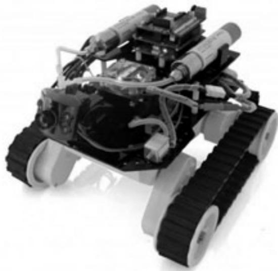
Horizon's HYDROSTIK PRO hydrogen gas-absorbing metal hydride cartridges – these are in turn refilled using the included HYDROFILL PRO desktop hydrogen station, which extracts hydrogen from water stored in an integrated reservoir.
