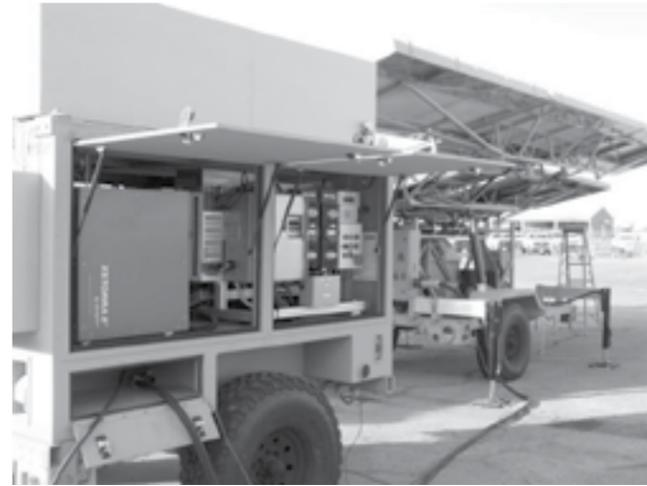
lab at China Lake, California, prior to field testing with troops. NAWCWD Renewable Energy Office electronics engineer Matt Malone says that the new fuel cells can be towed to remote locations to produce energy using water and sunlight. Designed to be deployed anywhere, the new environmentally friendly renewable energy system features recyclable fuel cell and an array of solar panels. It is capable of generating around 5,000W of electricity.
