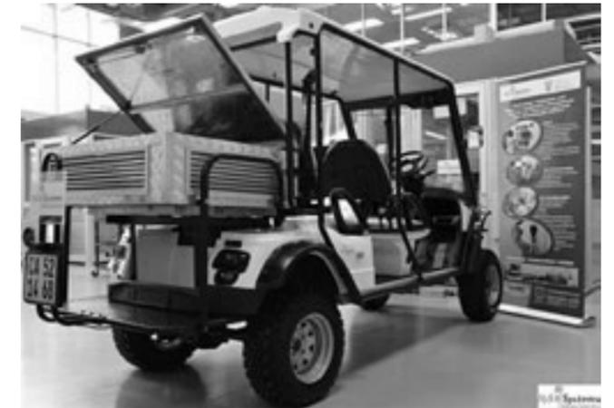
A team at the University of Western Cape's dedicated hydrogen systems center have been testing the efficiency of the fuel cell cart to see if it performs better than the campus's current fleet of diesel and battery-electric vehicles. Professor Bruno G Pollet and team at Western Cape's Hydrogen South Africa (HySA) Systems Competence Centre said the addition of the fuel cell to the cart saw its range double as well as it reaching a top speed of 30mph.
